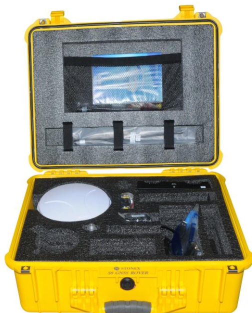
Fig. 3.2 - S8 internal case of Rover
