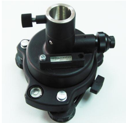
Fig. 3.15 – Tribrach and adapter with optical plummet
