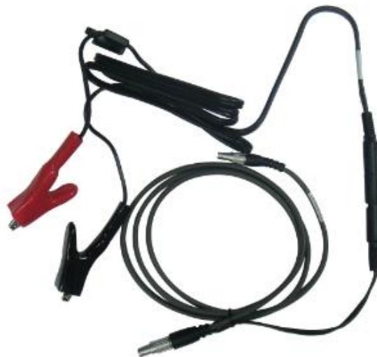
Fig. 3.10 - External power supply cables
